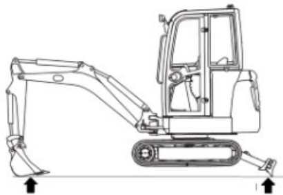
Figuur 6.14 Machinestand controle spanning rupsketting
