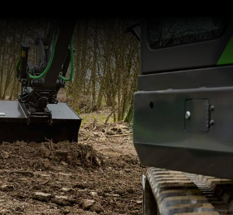
Since 2022, Volvo Construction Equipment has held a majority stake in Limach. This collaboration between the two manufacturers brings a new focus on efficiency and sustainability. The base machine is produced by Volvo without diesel components and delivered as a semi-finished product to Limach's factory, where it is completed as a fully electric machine. This eliminates wasted time and materials. A jointly developed concept is now available to you: Volvo quality, Powered by Limach!
